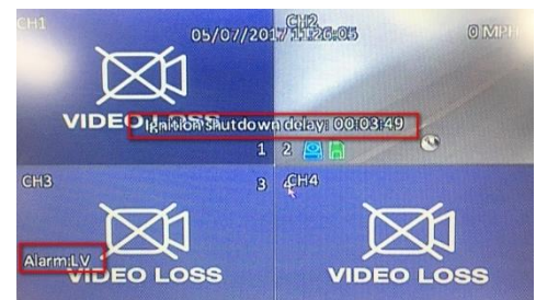
Low Voltage Shutdown Delay Figure 36
