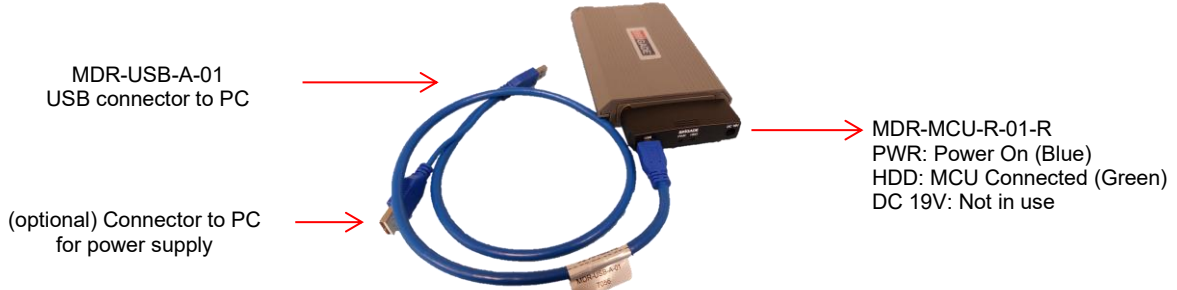
MDR-641-X-MCU-XXX Connection with MCU Reader Figure 4
