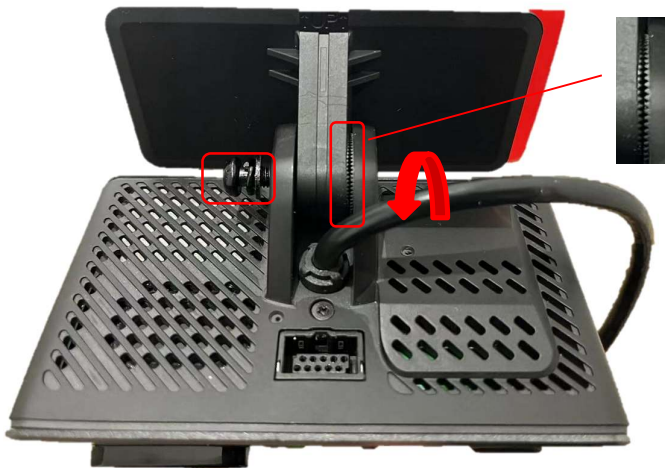
Picture showing the fixing screw, angle of rotation of DC-204-AI Figure 12
