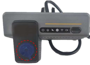
DC-204-AI Front view showing LEDs and button and driver facing lens of DSC camera Figure 10
