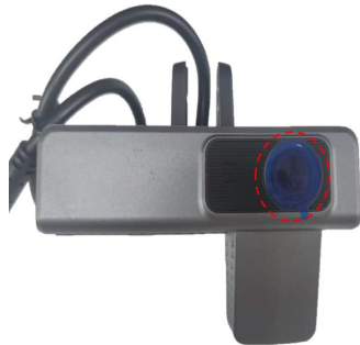
DC-204-AI Rear view showing the road facing lens of the ADAS camera Figure 11
